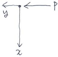
$$y = e^{\beta x} (C_1 \cos \beta x + C_2 \sin \beta x) + e^{-\beta x} (C_3 \cos \beta x + C_4 \sin \beta x)$$
